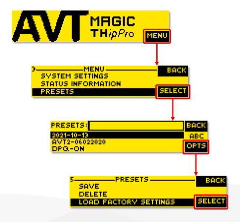
If there is a password configured but the password is not known, the device can only be reset via front display as shown on the right.
